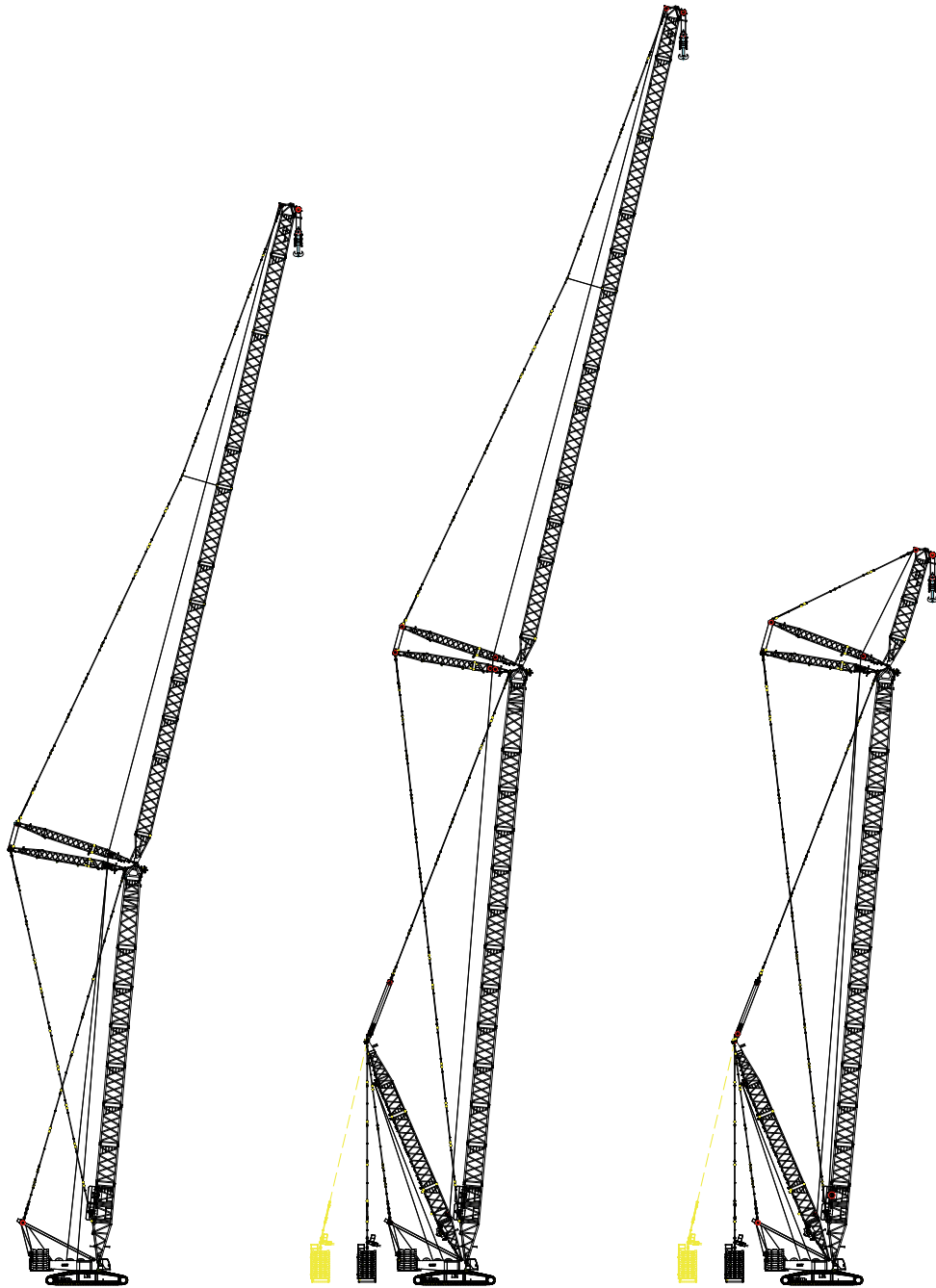
LJ Operating Condition Boom: 36m-60m Luffing Jib: 30m-102m
